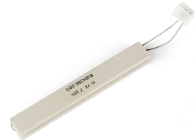
Fig. 18: Wire-wound resistor assembly for power supply load testing.
