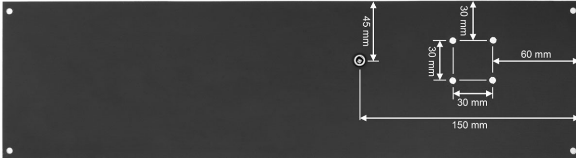
Fig. 62: Drill hole positions for the power supply board on the back panel. This is the view from the outside face of the cover (the power supply board is later to be placed on the opposite side).
