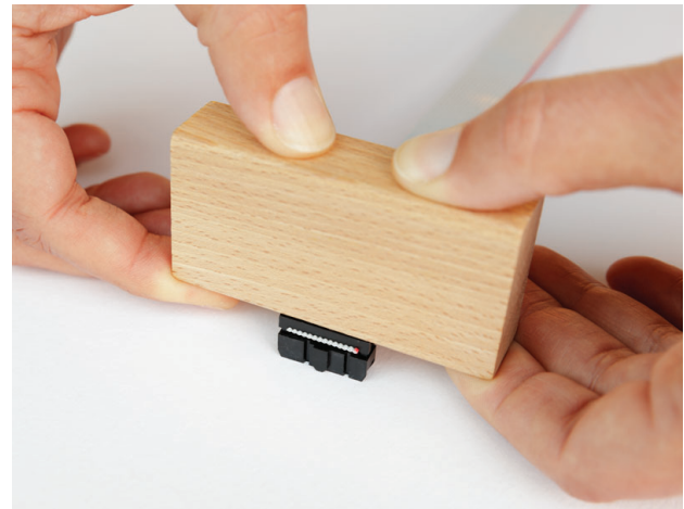
Fig. 8: Apply pressure evenly on each wire-to-board connector.
