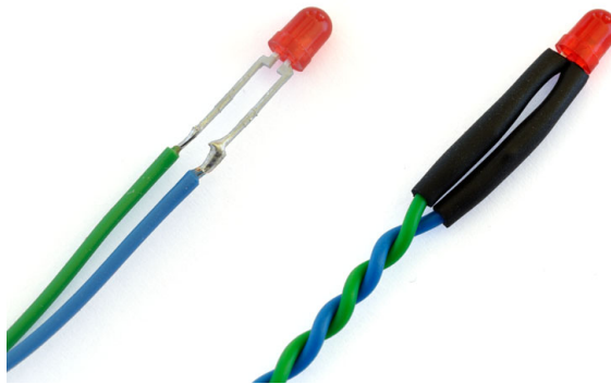
Fig. 12: Front panel LED assembly, on the right with the shrink tubing added.
