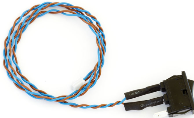
Fig. 14: Front panel switch assembly. Unlike shown here, you should also isolate the unused lead. If a cable ever comes loose somewhere in the build, it helps avoid inadvertent contact to an unused lead.
