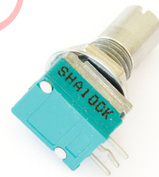
This pot fits the board's footprint well but its thread is too long.
